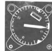
Pointer at or below lower edge of approach index marker
