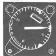
Pointer near center of approach index marker
