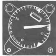
Pointer just above center of approach index marker
